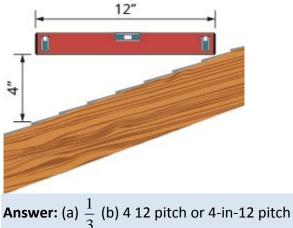
280. The slope of the roof shown here is measured with a 12" level and a ruler. What is the slope of this roof?
