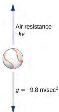
Figure 4.24 Forces acting on a moving baseball: gravity acts in a downward direction and air resistance acts in a direction opposite to the direction of motion.
