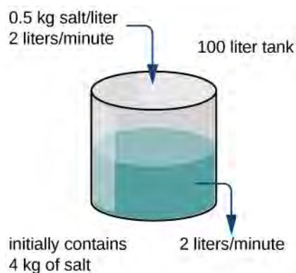
Figure 4.16 A brine tank with an initial amount of salt solution accepts an input flow and delivers an output flow. How does the amount of salt change with time?
